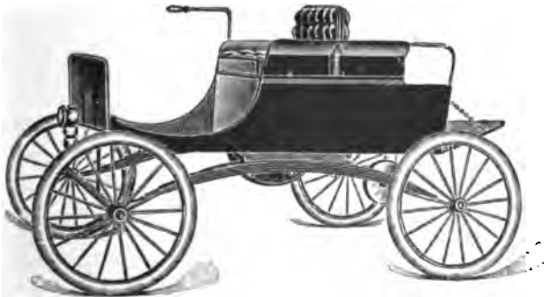
FIG. 74a.—An American Gasoline Vehicle, equipped with side spring frame, after the fashion of several models of horse carriage. This style of underframe is very suitable for light motor carriages, overcoming many of the disadvantages of the usual spring constructions.
